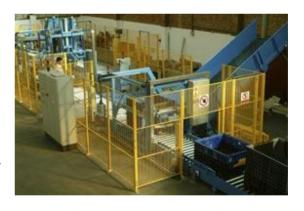
The works cycle begins with the parts being removed from the containers, leaving only packaging waste such as dunnage, cardboard and plastic in each unit. The container then travels along a conveyor until it reaches a machine module where a special frame assembly grabs and lifts the container and positions in over an adjacent belt conveyor that serves two compacting machines. The assembly then automatically pivots to tip the container and release the waste ready for compacting and disposal.
