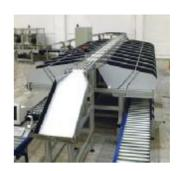
Axiom GB Ltd has launched its high speed Series 25 sorter as the latest product to emerge from the company's ongoing research and development programme. The new Series 25 sorter sets the standard for versatility and performance. Not only capable of accommodating different sized products – from credit card size up to cartons and boxes weighing 30 kg – it can also be easily configured to suit an almost limitless range of different applications.
