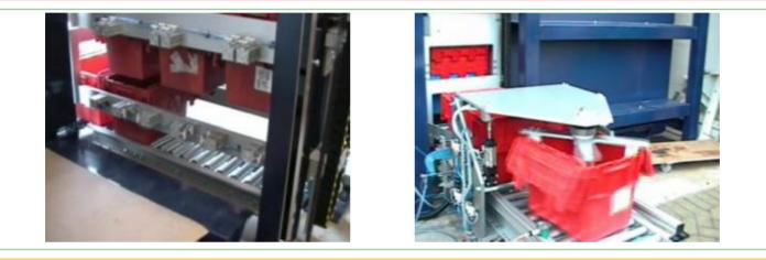
Palmers needed a solution for automatically de-stacking returned totes onto a sorting system at one every three seconds. The totes had to be rotated as necessary to ensure that an imbedded RF tag was always presented in the correct manner to the filling machines.
