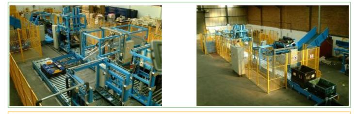
In a quest to increase productivity Ford recently installed an automatic container handling system at its Cologne plant that supports production of the Fiesta range.
